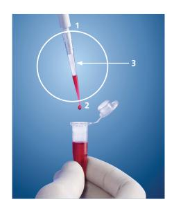
There are two different types of pipettes: air interface and positive displacement. Air-interface pipettes are usually used for the exact pipetting of aqueous solutions in the ml and µl range. For media with high vapor pressure or high viscosity, positive displacement pipettes are used. The
