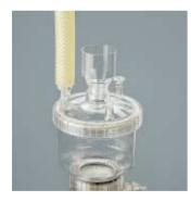
Type 16511 is like 16510, but without receiver flask. It is used on a suction flask or a vacuum manifold, e.g. Combisart, page 32.
