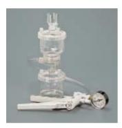
For sterile filtrations, the filter holder, comprised in the delivery, is equipped with a glass fibre filter 13400-0013 and enables a sterile venting for pressure compensation in order to avoid contamination of the sterile filtrate. The funnel fits onto the central opening of the lid and simplifies the pouring-in of liquid in the top part.
