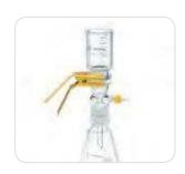
All areas, where liquid and device can come into direct contact, are made of glass or PTFE. The device, in combination with solvent-resistant, hydrophilic RC-membranes, is therefore ideal for ultracleaning and degassing solvents and solvent mixtures for HPLC, GC and AA. Convenience of handling is ensured by several beneficial features. A 6 mm wide
